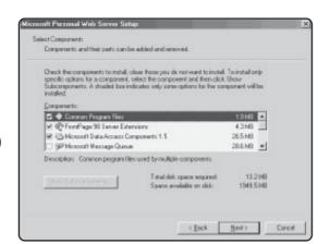
Be sure to select only the necessary components for installation of the PWS.
